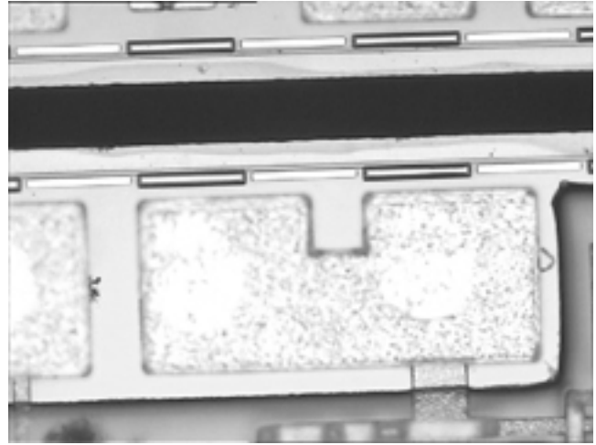
Fig.6. 26 μm cut in 100 μm thick GaAs
