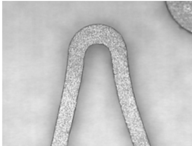
Fig. 2. 200 \mu\text{m} thick and 120 \mu\text{m} width Nitinol stent cut with the Laser Microjet (no further process)
