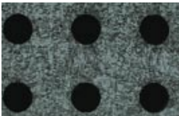
40\mu\text{m} diameter apertures in a 40\mu\text{m} thick stainless steel sheet. In this case the cutting speed is equivalent to 40,000 holes per hour.
