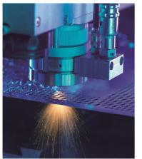
Water Guides the Laser - The application becomes insensitive to the focal plane of the laser. A cylindrical laser beam is created resulting in perfectly parallel walls, tight kerf widths and enabling the user to cut thick or non-flat parts, without having to worry about being in focus.
