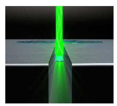
The cutting kerf width ranges from 25 to 120  $\mu$ m, depending on the nozzle size. The laser energy is always guided to the bottom of the kerf.
