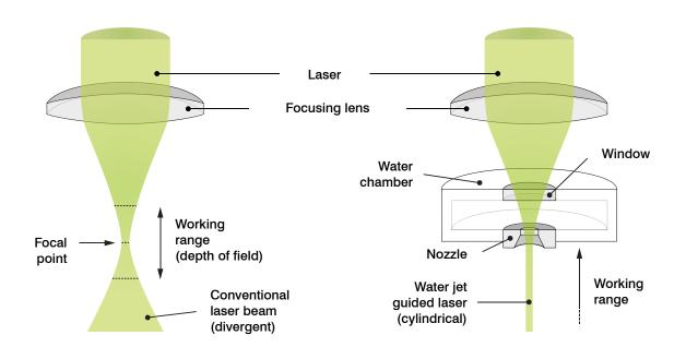
The conventional focused laser beam has a limited working distance of just a few millimetres to even fractions of a millimetre due to beam divergence.
