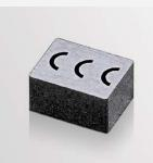
Micro-Machining: Spinnerets. Cutting of 4 mm stainless steel: 7 min/slot
