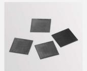
Lab-grown Diamonds: Slicing of 10 mm CVD diamond in 15 min
