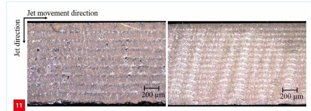
Comparison of the kerf surface of a 1.4-mm-thick silicon sample machined with the multi-pass strategy; left and right with different laser power and process speed values (see the text).
