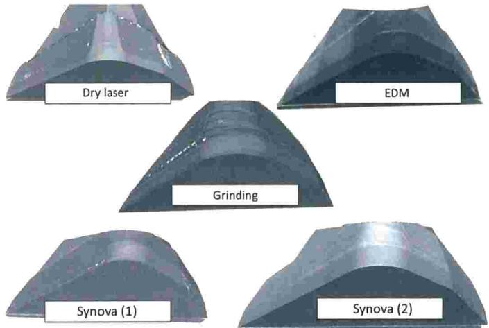
In the above example, the Synova LMJ (1) process took twelve minutes to cut the entire workpiece to final dimension and quality while the Synova LMJ (2) process took 16 minutes. The other machining technologies take similar processing times.
