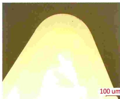
SCD tools represent the wave of the future and Synova's LMJ technology allows single crystalline diamond material to be machined with virtually no heat affected zone. Thus, a standard single point cutting tool retains its material qualities within its geometrical profile.
