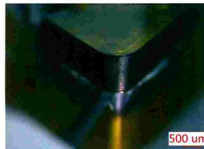
Such a high quality of surface finish is proof that the LMJ technology is best suited for the laser machining of SCD tool inserts. While cutting trenches are visible on the SCD insert, here brazed on to a holder, they have no impact on the surface roughness achieved on the workpiece.
