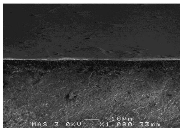
The flank is very smooth. There is some slight contrast produced showing how the laser scanned back and forth. The scan lines indicate how much material is removed with each pass
