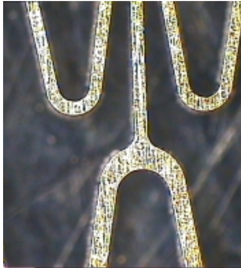
Detail of stent cut with Laser Microjet Process, 40 x magnification
