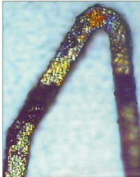
A cut with a conventional laser shows thermal damage on its backside, and has a rough edge.
