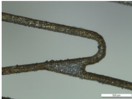
Figure 11: Microscopic image of a 316L stainless steel stent cut with dry laser, directly after cutting.
