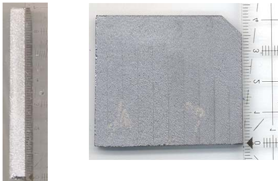
Fig. 3: Silicon wafers cut off thick Si plates via LCP (with water as carrier liquid) using a high-power ms-pulse laser. The liquid jet was orientated vertically in the pictures so that the cutting depth was 7 cm (left) and 4 cm (right).
