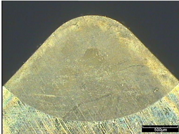
Fig. 11: Microscopic view of front side showing the CBN insert
