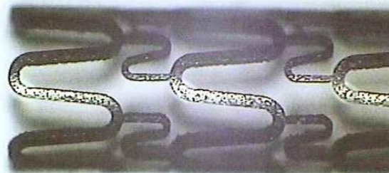
FIGURE 4. Close-up of stainless-steel tubular stent cut with the Laser MicroJet from 1.5mm diameter tube.
