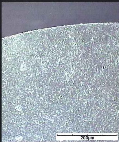
Photo 6 – EDGE OF A CBN CYLINDER (diameter: 3mm) directly after cutting with the Laser Microjet
