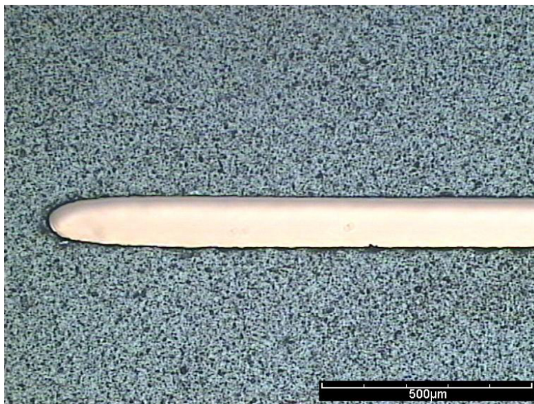
Figure 6 – Slot start in thick silicon (backside)
