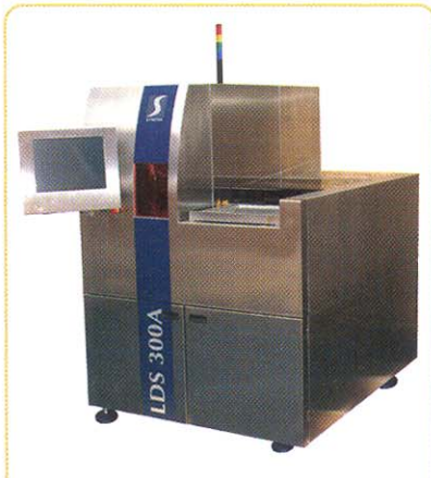
Figure 1. The LDS 300 is Synova's newest laser dicing system (LDS) based on its innovative water-jet-guided laser technology. Designed to provide chipmakers with a high-speed tool with a large working area, the LDS 300 allows cutting for up to 300-mm wafer size and dices chips down to 0.25 x 0.25 mm. Footprint of this fully automatic dicer, which includes wafer cassette loading, cleaning and quality control, is the smallest on the market (1.75 m 2 ).
