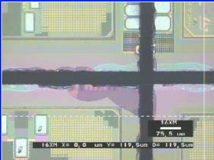
Typical chipping and delamination of low-k layers due to abrasive sawing
