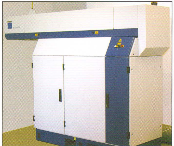
Figure 3. Infrared Trumpf laser coupled in water for stencil cutting.
