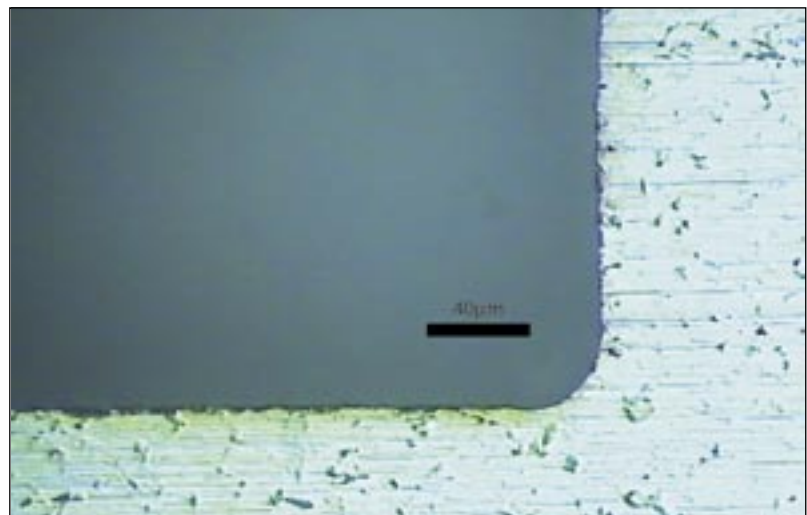
Figure 5 - A corner of an aperture at higher magnification. The jet diameter was 40 \mu m as indicated by the scale-bar
