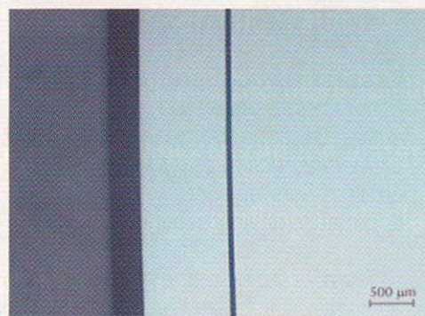
Microscope image of the grooving in a thick silicon wafer, before back-grinding.
