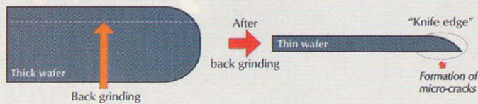
Back-grinding of thick wafers creates a "knife edge."
