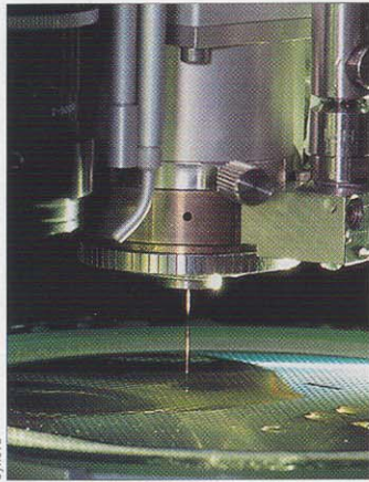
Synova says that its water-guided laser is suitable for cutting metal stents and stencils, or slicing silicon wafers.
