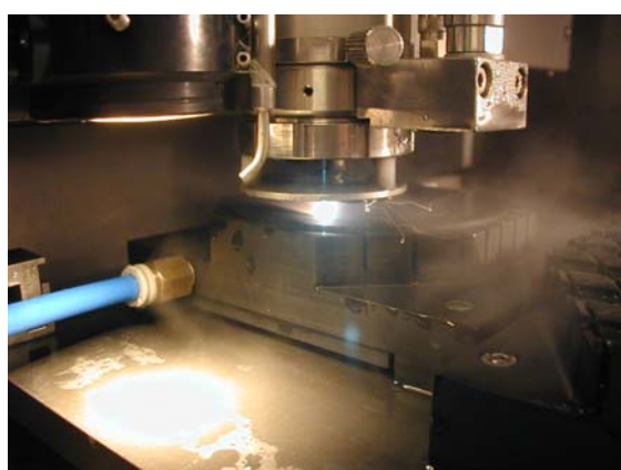
Fig. 4: The LMJ in action cutting a CBN disc on a special vacuum chuck designed for this application.
