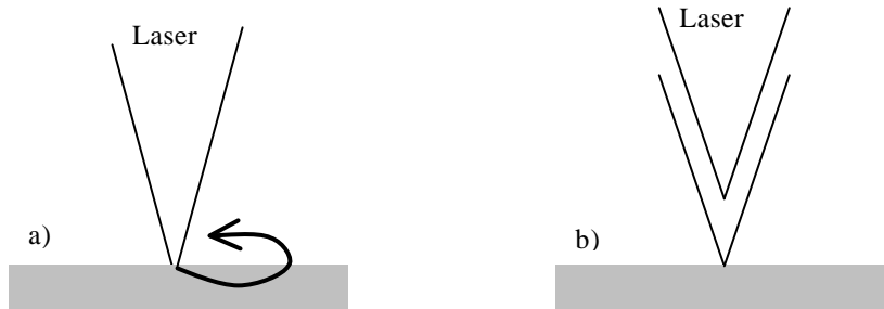
Figure 6: Schematic of trepanation drilling (a) and percussion drilling (b)
