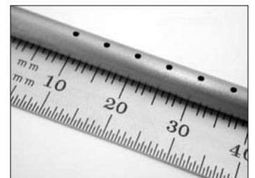
Figure 7. Holes (0.9 mm) in the side of a pipe, drilled with the laser Microjet.
