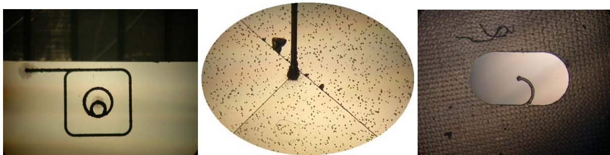
Figure 4. The strong initial laser pulse forms a crater and might break the wafer.
