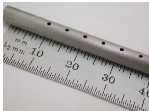
Fig 5: Left: with Laser Microjet cut vacuum grip. Right: Holes (0.9 mm) in the side of a pipe, drilled with the water guided laser.
