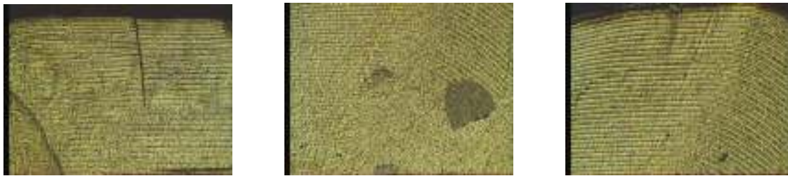
Laser- Microjet® cut Diamond, cut surface, magnified (10x)
