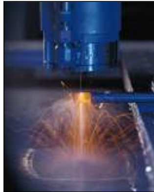
Cutting with water jet guided laser
