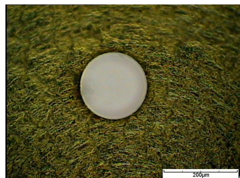
Highly magnified back surface view of Injection Nozzle hole
