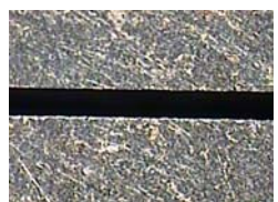
Perfect cutting with the water jet guide laser (100x)
