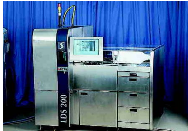
LDS 200 A (Fully Automatic Laser Dicing System)
