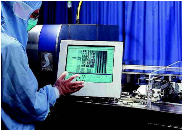
LDS 200 A (Fully Automatic Laser Dicing System)
