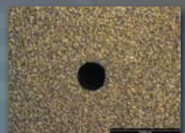
Si solar cell Cutting speed per hole: 2s Hole diameter: 210µm
