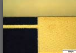
Mono crystalline Si solar cell Cutting speed: 125 mm/s Thickness: 230µm
