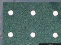
Polycrystalline solar cell Cutting speed per hole: 1.8s Hole diameter: 100µm
