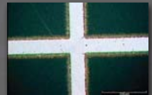
CIS + Mo on glass, groove width ~70µm Electrical isolation R>20MW Cutting speed: 500 mm/s
