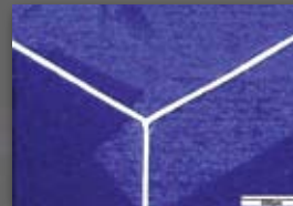
Hexagonal Dicing of Si Cell 4" wafer hexagonal shape 900 chips/wafer Throughput: 1.67 s/chip
