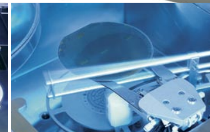
An automatic handling system in the LGS allows for safe wafer transfer to the next manufacturing step – cleaning with either high pressure water or using a megasonic system. This, combined with the tool's small footprint, makes the LGS an easily integrative tool into any production line.
