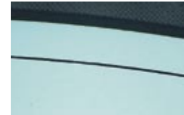
After back grinding, thin wafers are very brittle. Their edge contains micro-cracks due to the thinning process, making them subject to breakage during handling. Removal of the wafer edge, using a gentle technology, increases the wafer strength.
