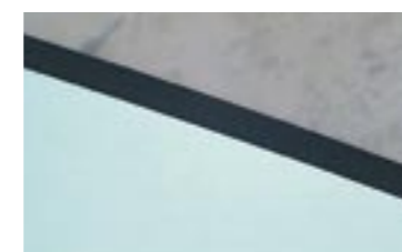
The edge of this 625-µm thick silicon wafer was 75-µm deep, trimmed at a width of 300 µm. This approach prevents a sharp edge from forming after back grinding. The operation takes only 240 seconds for 8-inch wafers and 300 seconds for 300-mm wafers
