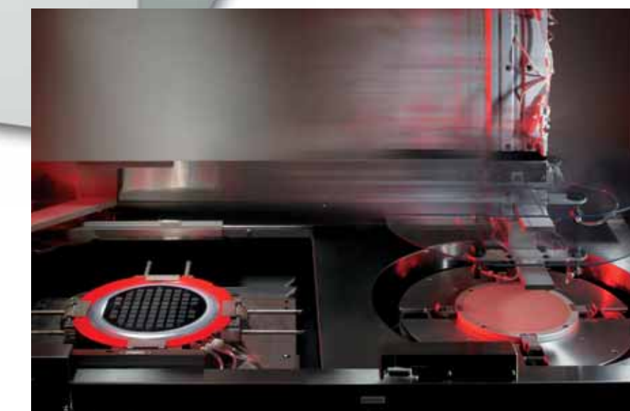
The frame pick arm moves the workpiece from the cassette to the pre-alignment stage which, after centering, is moved to the chuck table for cutting. After cleaning and drying at the spinner table, the workpiece is returned to the cassette.
