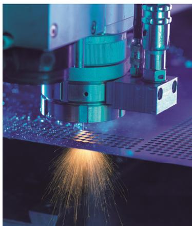
**Water Guides the Laser** - The application becomes insensitive to the focal plane of the laser. A cylindrical laser beam is created resulting in perfectly parallel walls, tight kerf widths and enabling the user to cut thick or non-flat parts, without having to worry about being in focus.
