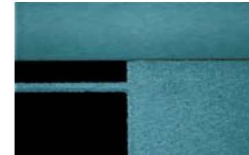
Another application is through cutting or edge isolation of silicon PV solar cells. Grooving speeds reach 300mm/s. This 350-µm thick cell was completely cut at a speed of 80 mm/s.
