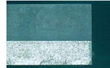
The LCS is Synova's most versatile machine. One of its applications is cutting of hard materials for the tooling industry. This 1.6-mm thick insert, consisting of two layers – CBN and WC-Co, was cut in 20-30 mm/min. Edges are smooth and clean. The obtained edge surface quality is better than that obtained by EDM.
