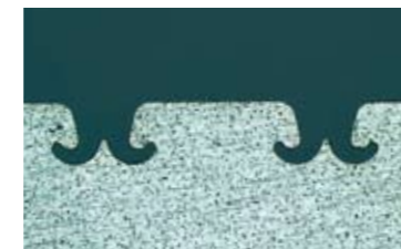
The Laser MicroJet® is an omni-directional tool: any shape can be created. This complex design was achieved at 2 mm/s in a 150-µm thick stainless steel sheet.
