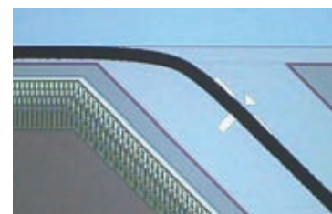
A 725-µm thick silicon wafer cut for a X-ray image sensor chip. The through-cut is clean, chip-free and smooth. Absolute sensor surface cleanliness can be achieved without using a protection film.
