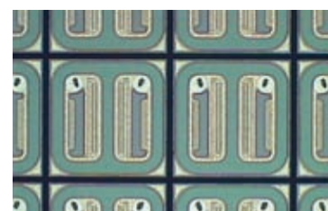
A silicon wafer diced with a 50-µm kerf. A fully automatic kerf check ensures maximum precision.
