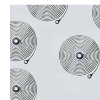
Precision Parts – Watch Spring 130µm thick, 50µm wide silicon 10 mm/s cutting
