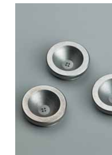
Automobile – Fuel Injection Nozzle 160µm stainless steel 3 mm/s cutting/2.5 seconds per hole
