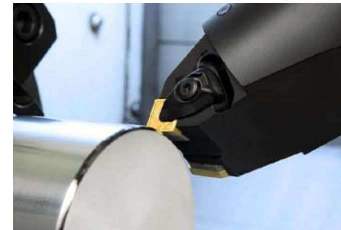
Hard Tooling : Super hard material such as cubic boron nitride (CBN), polycrystalline diamond (PCD), silicon nitride (SiN)
